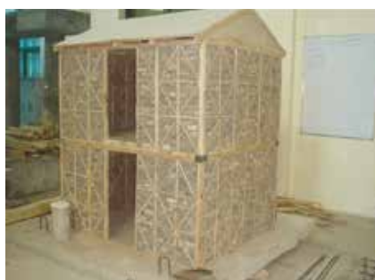
Reduced scale model of a Dhajji house on the shake table of the Earthquake Engineering Centre of the NWFP University of Engineering and Technology Peshawar, Pakistan
